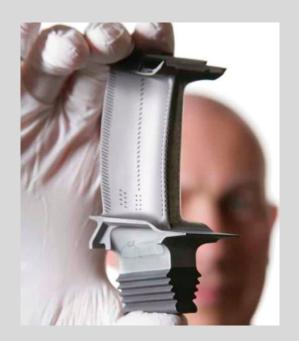
We have even worked out ways to make crystals grow in the shapes we want them to like this part for a jet engine (could you grow crystals in a mould to make different shapes?)
