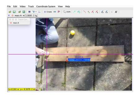
2. Change the graph x-axis to px(kg m/s) where p stands for momentum (in the x-direction) - hover the mouse over the label and choose from the list:
